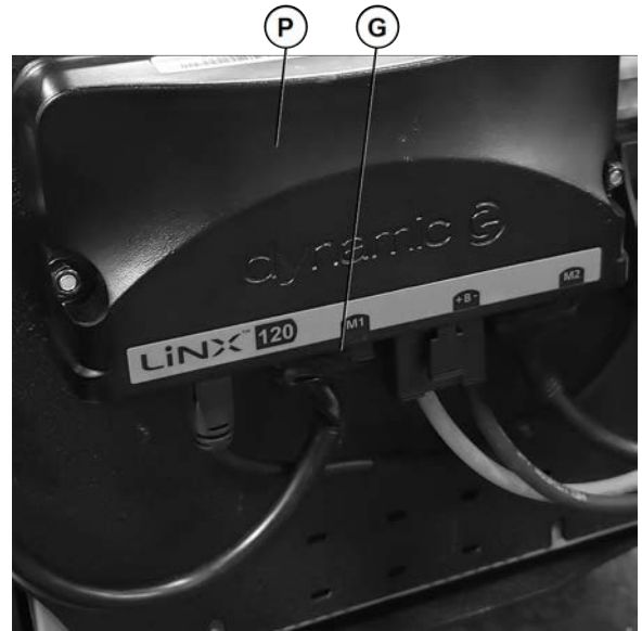
Fig. 10-5 Disconnecting the motor cable
