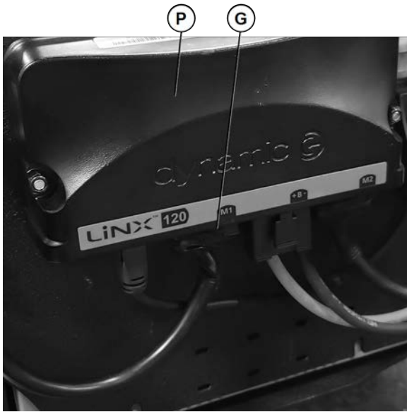
Fig. 10-8 Connecting the motor cable
