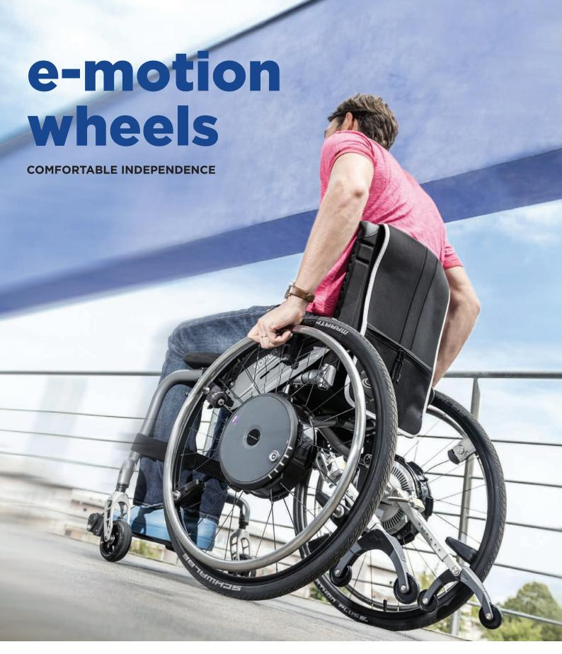
The concept of e-motion is ingeniously simple: While moving, sensors built into the push rims measure your drive movement and provide you with the desired motor power. This allows you to move, steer and brake your wheelchair with very little effort. With a weight of only 7.8 kg per drive wheel, e-motion is one of the lightest active add-on drives available
