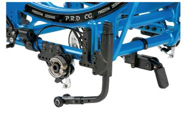
Stainless steel tilt mechanism with easily visible tilt angle identification.
